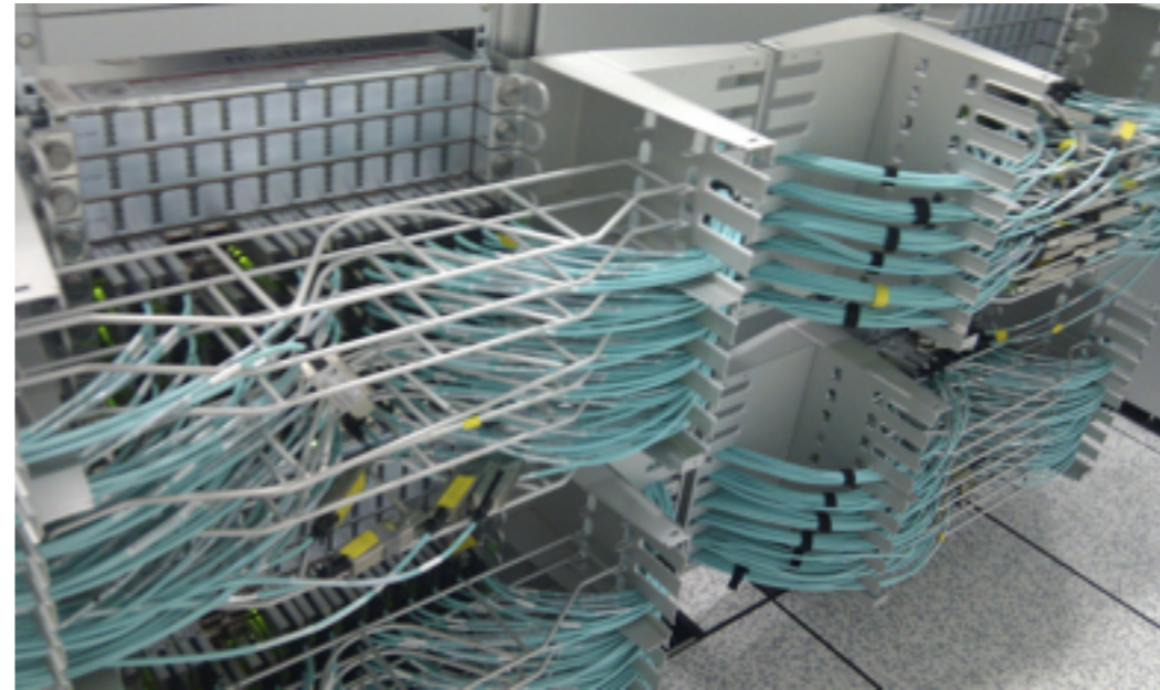
Infiniband interconnect: up to 30,000 computers via MPI
