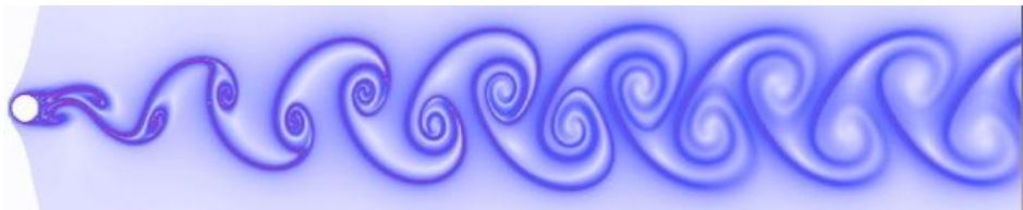
Lagrangian perspective (FTLE): Highlighting separation of particles FTLE: finite time Lyapunov exponent
