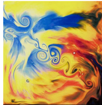
Mixing of a fluid – color pH value of fluid. CAP Arts of Physics, vis thymol blue.
